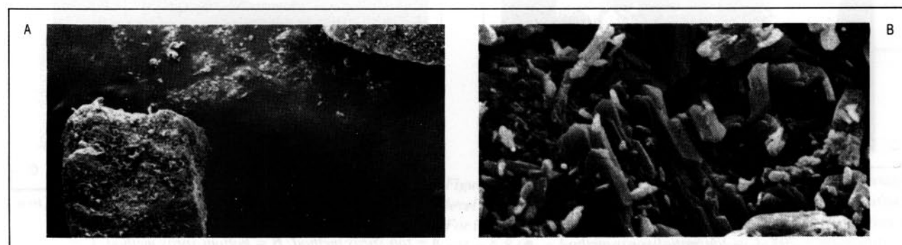
Figure 12: Surface of uncoated aspirin granule (A: magnification = 41X; B: magnification = 1000X).
